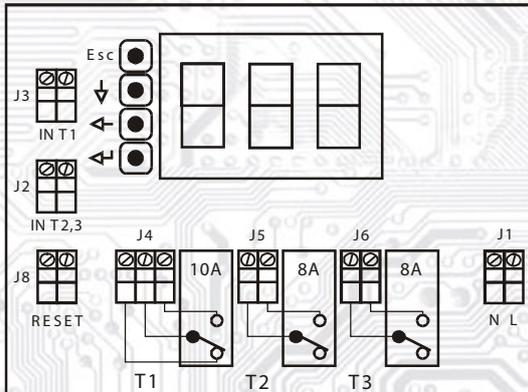
The relay contacts are illustrated in the still-stand position, which corresponds to the supply voltage switching off.
